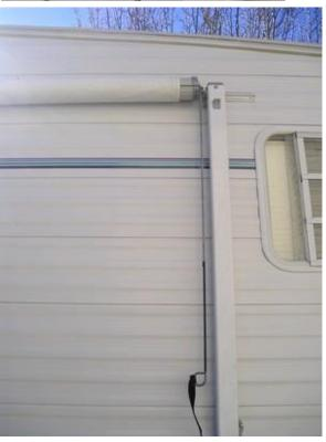
The lower end of the rod can be wrapped with electrical tape to keep from scratching the support arm.
