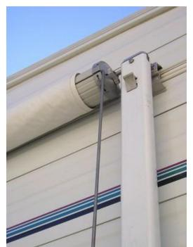
Insert the awning pull rod into the hole in the end of the roller tube.
