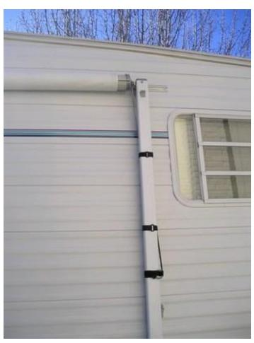
The rod is wrapped around the support arm and secured with velcro straps. Besides locking the roller it provides a place to store the rod.
